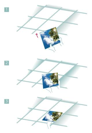
Refer to the image layout plan for proper placement. Direction arrows and numbers are placed on the back of each panel and on the corresponding layout plan.
