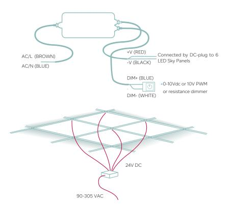
All LED Sky Ceiling and LED Wall panels are supplied as on/off (non-dimmable) as standard. We can also supply various types of dimmable LED drivers (DALI, Push-Dim, 0-10v etc.).
