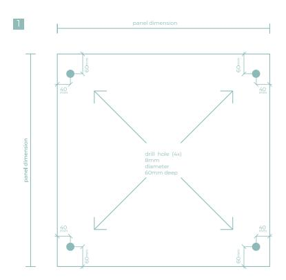
Drill the holes according to this drilling instruction.
