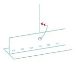
Squeeze grid hangers together if necessary to create space for the panels.
