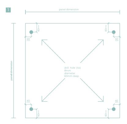
Drill the holes according to this drilling instruction.
