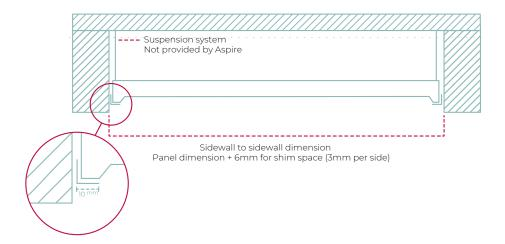
Recessed installations are as per the previous steps. However, as there is no grid system, a profile needs to be created for the panels. Please consult a skilled installer for the right materials and construction.
